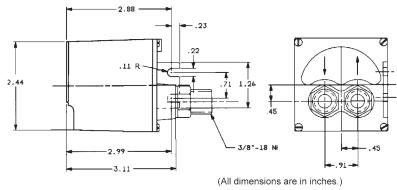
Connections are provided for attaching 3/8"- 16 NPT female fittings.
