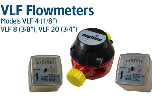
Red Seal Measurement VLF (very low flow) flowmeters have been designed to measure the flow of light fuel or diesel oil. They are available in three different sizes: 1/8" (VLF 4), 3/8" (VLF 8), and 3/4" (VLF 20) to measure flow rates ranging from 0.25 to 390 gph. The oscillating piston of these flowmeters forms two measuring chambers that are alternately filled and emptied. The passing oil is measured by fractions reflected by the register.
