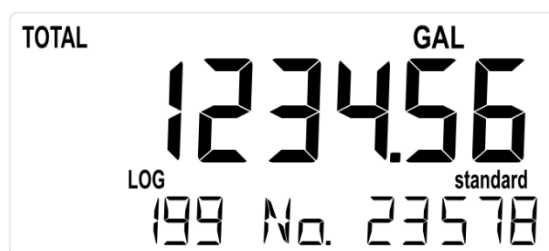
Fig. 14: Delivery record – corrected delivered quantity and delivery number
