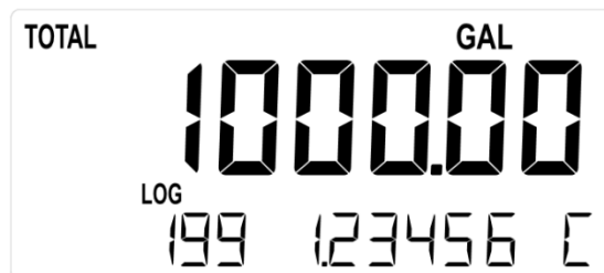
Fig. 21: Delivery record – uncorrected delivered quantity and average CTL
