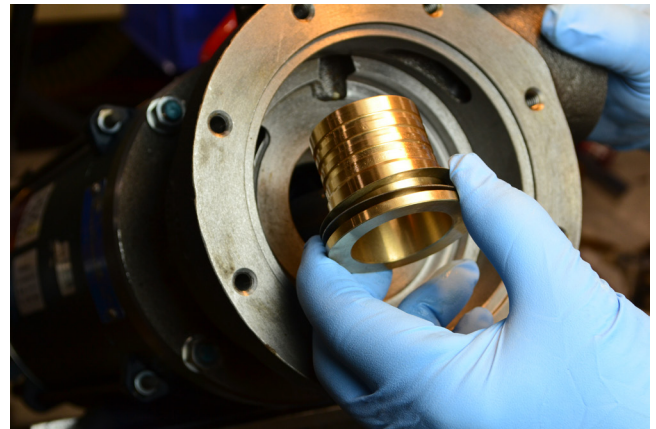
20. Place the shims over the housing. Note: during the following steps, be careful not to introduce foreign material or touch the seating surfaces. Rubber gloves are recommended.
