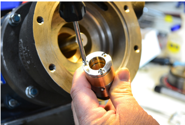
25. Remove the seal ring from the new seal and set aside in a clean location.
