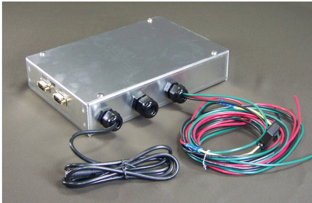
Figure 4-23. Junction Box Cables - Printer on Left, Truck Power on Right
