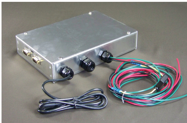
Figure 5-17. Junction Box Cables - Printer on Left, Truck Power on Right
