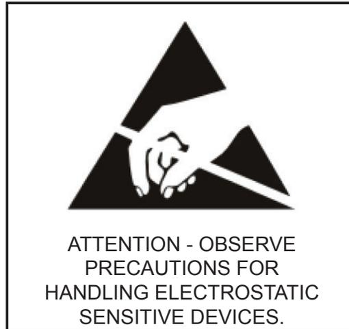
***Caution - This electronic device is sensitive to damage from ESD (electrostatic discharge). Observe the following precautions when servicing this device.***
