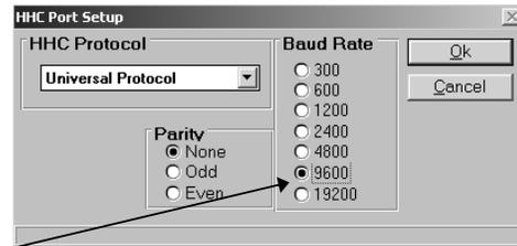
Also, make sure that the **HHC Port Setup** under the **Setup** Tab is in **9600-Baud Rate** (Default).
