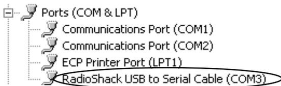
**Note:** In this example the diagram shows USB in COM3 Port. Computers without Communication Ports (E.g. some Laptops) will show COM1 or COM2.
