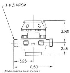
Connections are provided for attaching 3/4"-14 NPT
