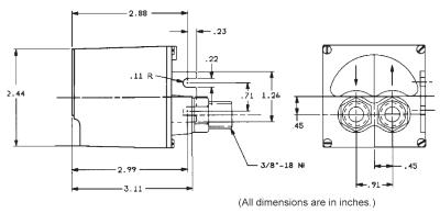
Connections are provided for attaching 3/8"- 16 NPT female fittings.
