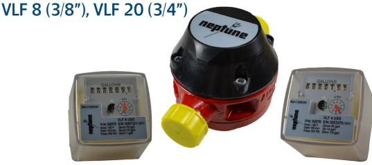
Red Seal Measurement VLF (very low flow) flowmeters have been designed to measure the flow of light fuel or diesel oil. They are available in three different sizes: 1/8" (VLF 4), 3/8" (VLF 8), and 3/4" (VLF 20) to measure flow rates ranging from 0.25 to 390 gph. The oscillating piston of these flowmeters forms two measuring chambers that are alternately filled and emptied. The passing oil is measured by fractions reflected by the register.
