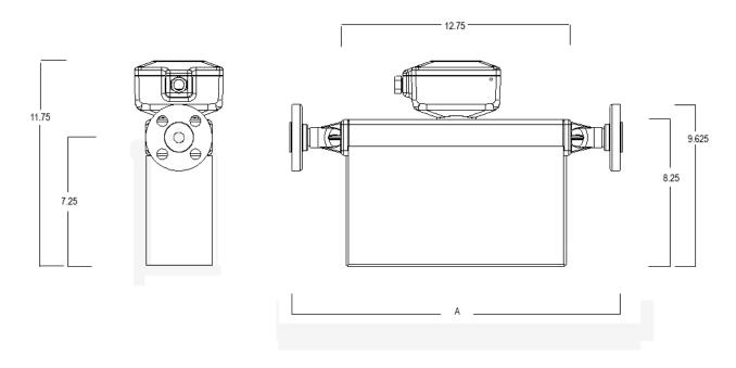
Shown with 1/2", 300# flanges and NexGen SFT200 Mass Flow Transmitter
